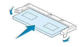
**NOTE**: If you have difficulty inserting the memory DIMM or closing the levers, make sure the notches on the bottom of the DIMM are aligned with the notches in the DIMM slot.
